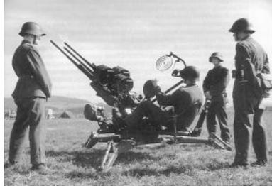
20 mm Flab Kan 43/57 Drilling (Hispano-Suiza)
